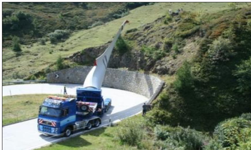
Plate 4-6 Blade adaptor transport system
